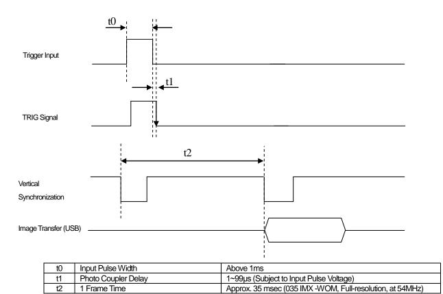
\*Trigger mode of 035IMX-WOM obtains images unsynchronized to camera capture cycle. To be specific, once the capturing process is finished, it initiates
